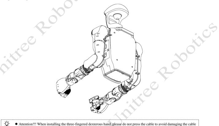
• Attention!!! When installing the three-fingered dexterous hand, please do not press the cable to avoid damaging the cable and causing poor contact!
